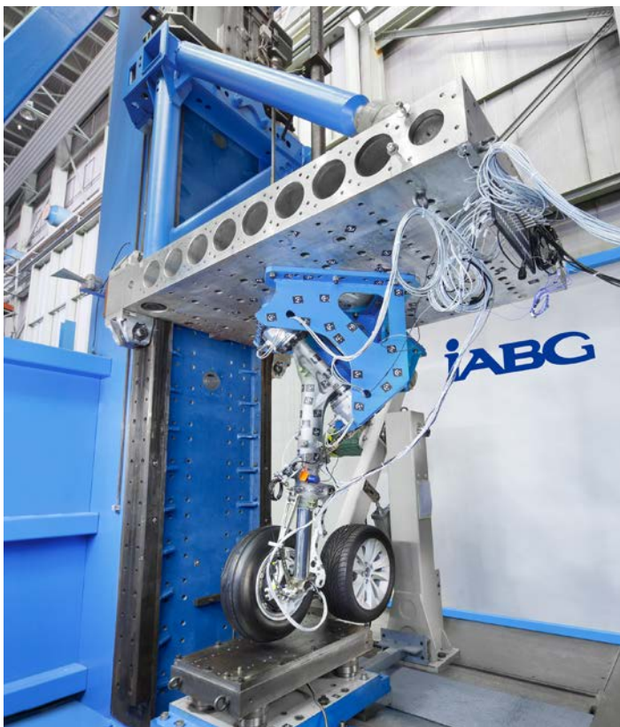
Functional test on landing gear (source: IABG).
