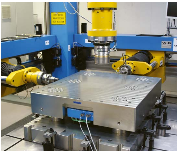
In-house calibration on Kistler's unique 3-component reference force press.
