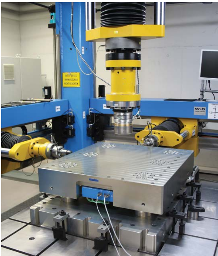
Calibration of a customized force dynamometer for the landing gear drop test on Kistler's special tri-dimensional calibration rig.
