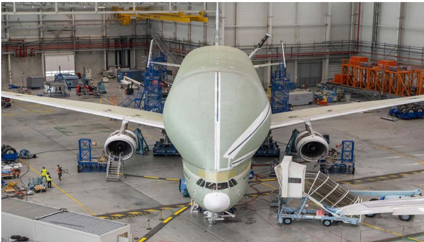
Prototype Airbus Beluga XL undergoes ground vibration testing (source: AIRBUS).
