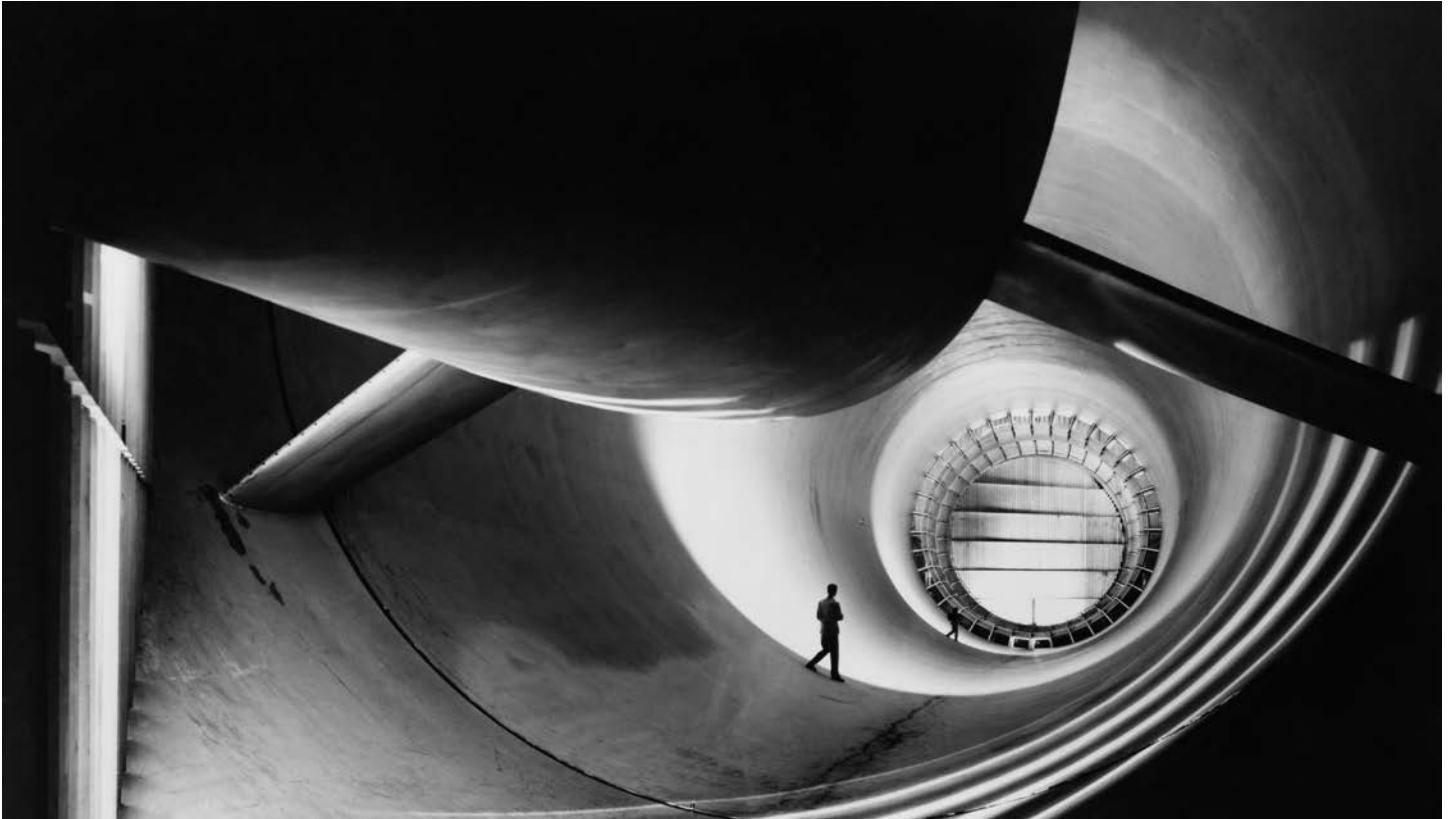
A wind tunnel is a tool used in aerodynamics research to study the effects of air moving past solid objects.
