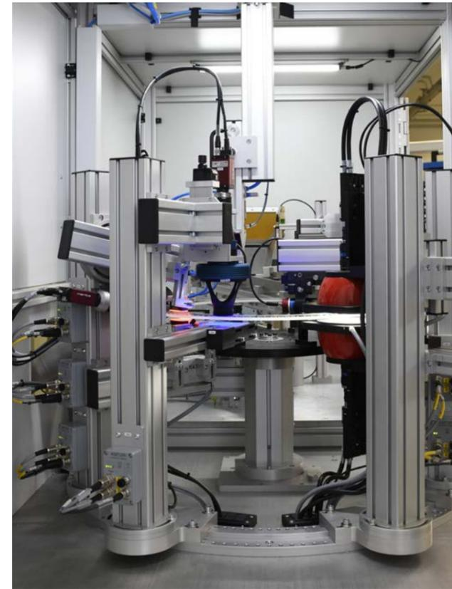
Modular setup with multiple camera inspection stations on a glass plate to inspect upper and lower sides of test objects
