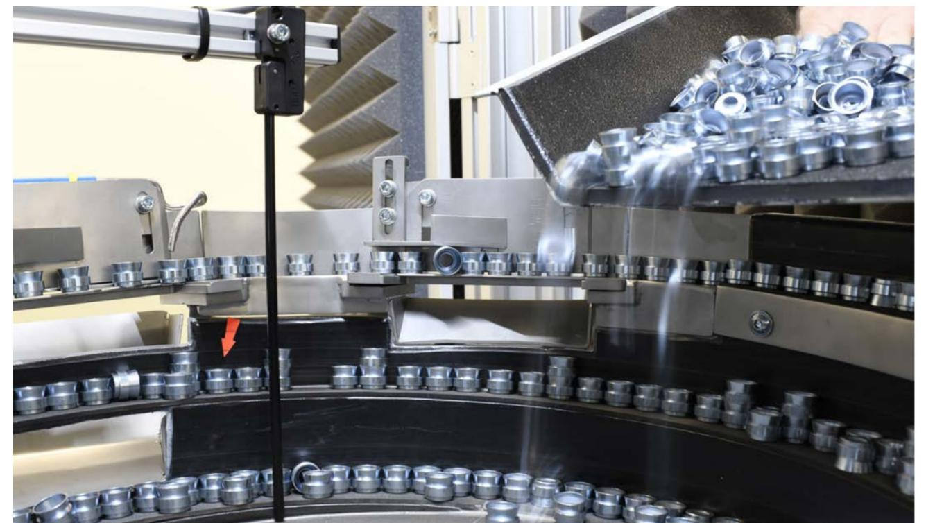
Modular conveyor unit for continuous feed of units under test
