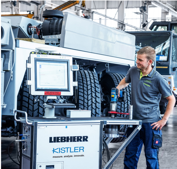
Testing related to fastening points on the Liebherr LTM 1450-8.1
