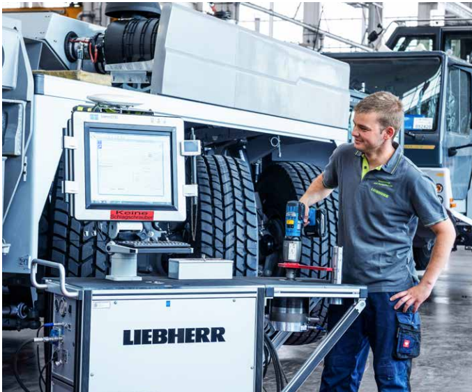
Testing related to fastening points on the Liebherr LTM 1450-8.1
