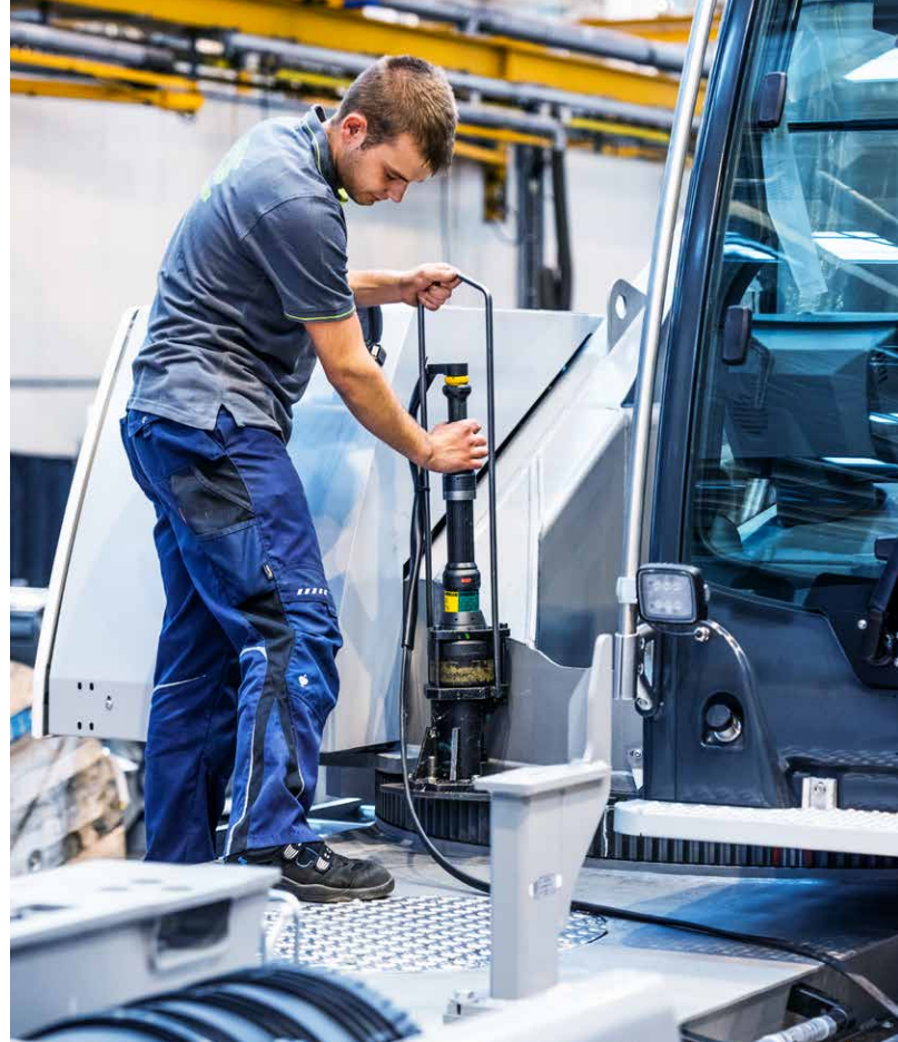
Fastening the slewing ring on the Liebherr LTM 1160-5.2, nutrunner: Atlas Copco ETDS9-2000-38-CTADS
