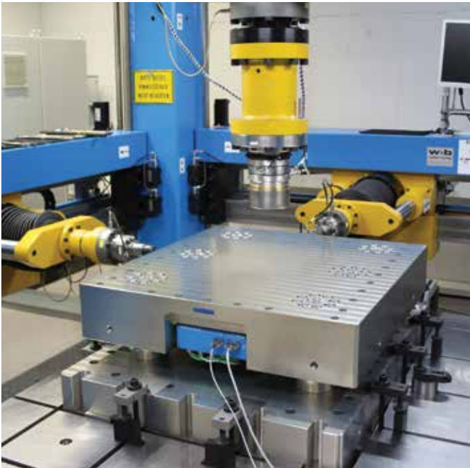
In-house calibration on Kistler's unique 3-component reference force press
