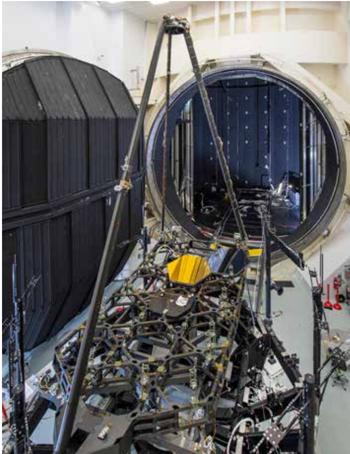
The full-scale James Webb Space Telescope pathfinder (test version of the backplane) shown going into NASA Johnson's huge Chamber A for cryogenic testing (Source: NASA/Chris Gunn)
