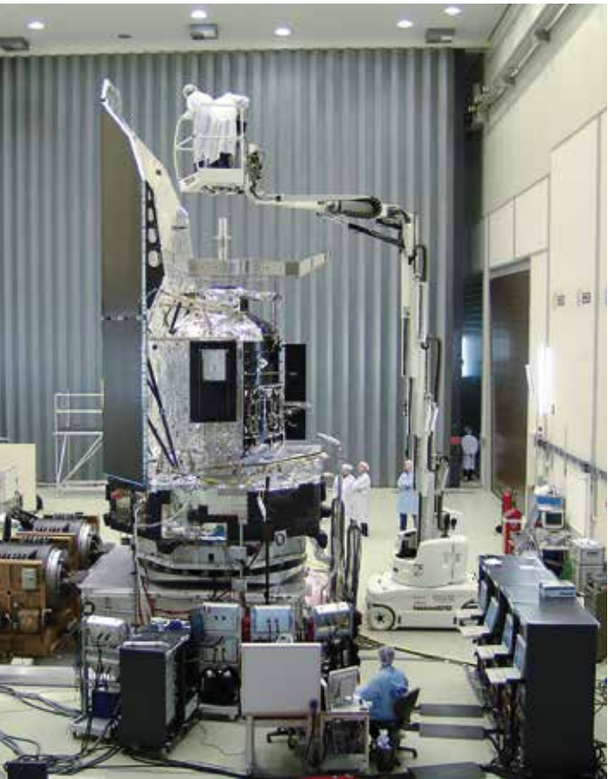
Environmental and ground modal testing of space structure (Source: ESA)
