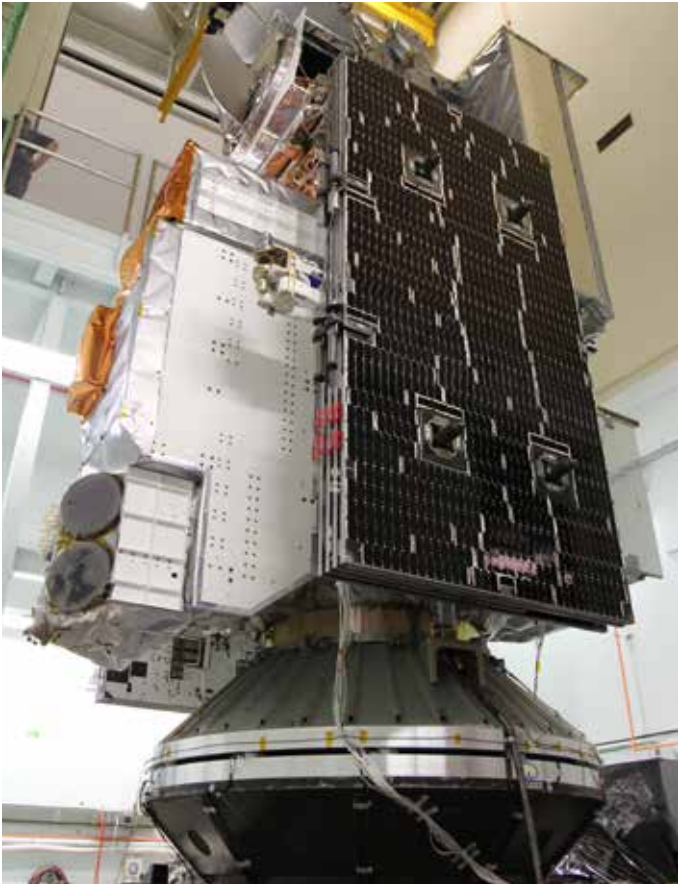
Satellite environmental vibration testing – Sine and Random vibration – (Source: NASA)
