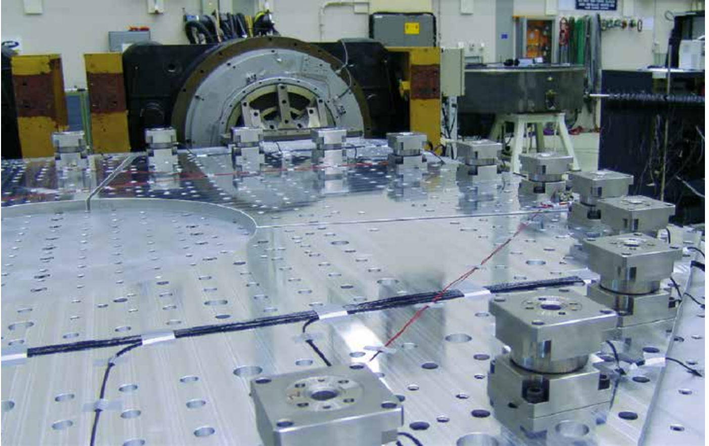
3-component force links mounted on the base plate, which is connected to the shaker. A force ring is then mounted to the load cell, which is sandwiched between the top and bottom ring. The space payload is mounted on the top ring for the FLV-test. (Source: ESA)
