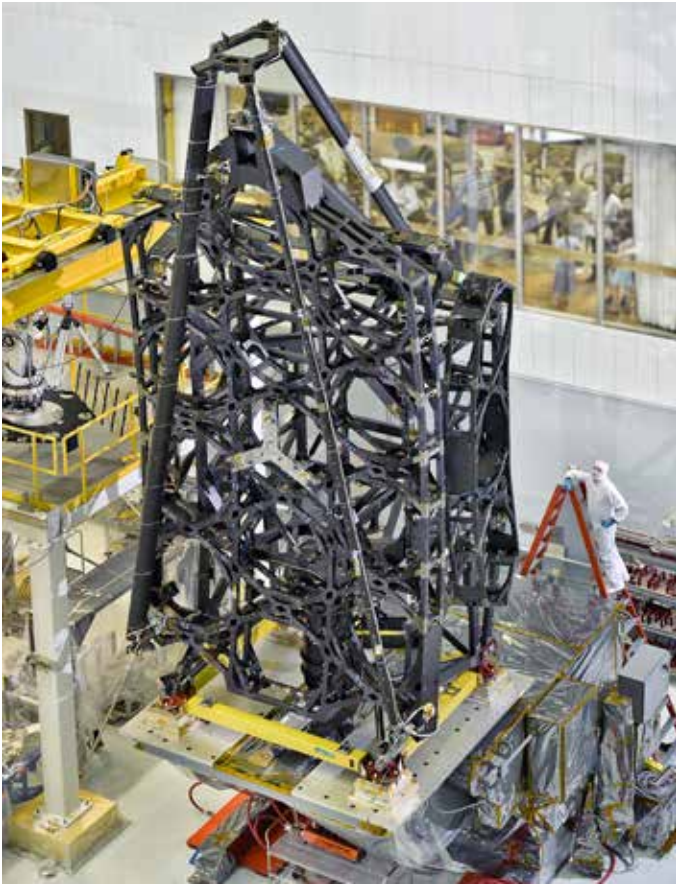
NASA's James Webb Space Telescope Structure getting ready to undergo thermal vacuum testing (Source: NASA/Chris Gunn)
