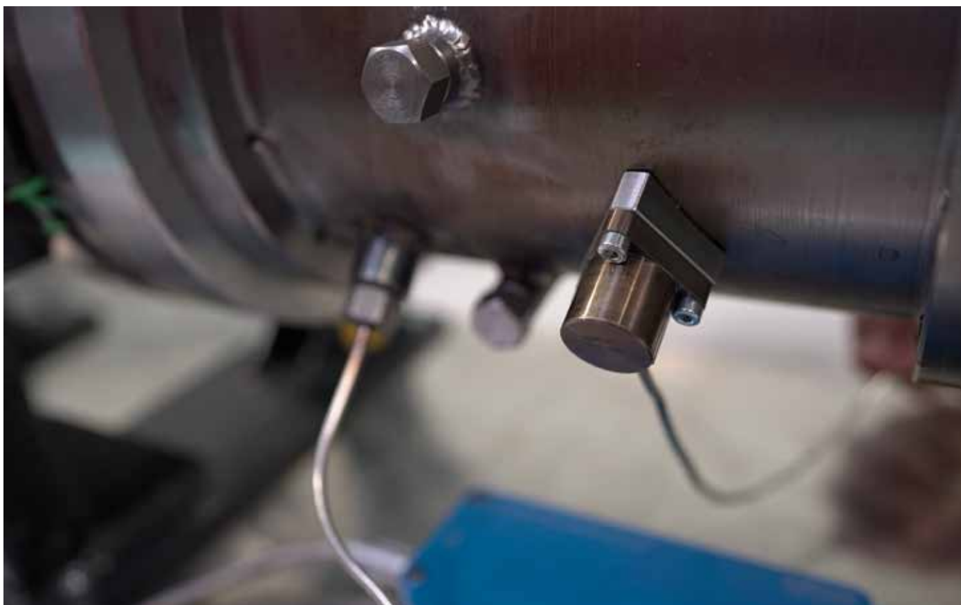
Combustion instability investigations use high-temperature Type 6021A pressure and Type 8209A acceleration sensors
