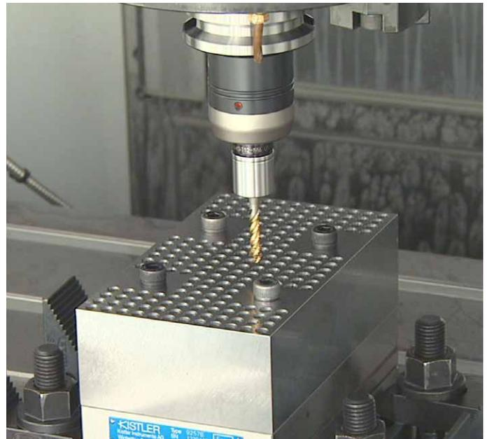
The tapping holder MEGA Synchro was developed with a dynamometer 9257B from Kistler
