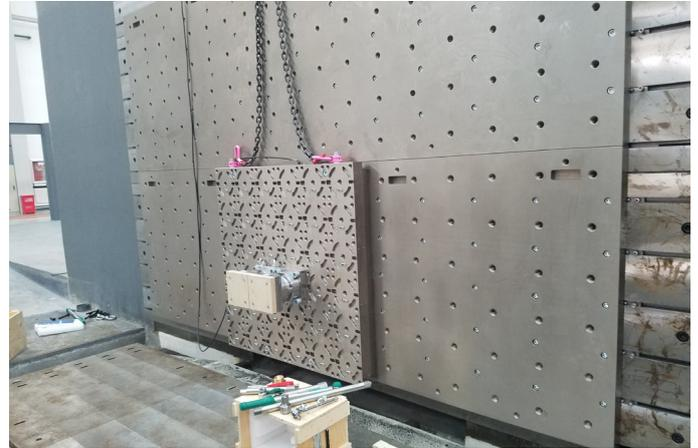
After an intensive engineering phase lasting several weeks, the measurement technology experts were able to develop a crash wall with a total of six segment plates
