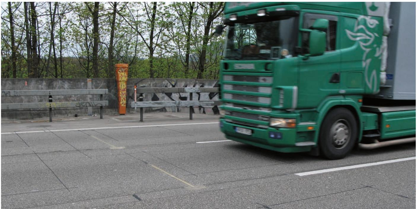
Calibration run with a reference vehicle.
