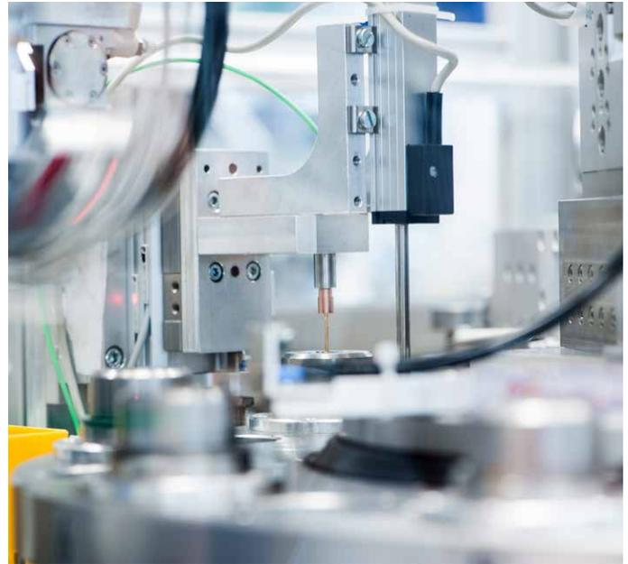
The last step in automated production is to verify the spring force of the probes.
