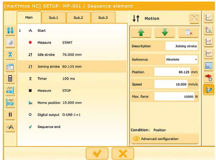
maXYmos NC actuates the NC joining module via the servo amplifiers for linear and rotary movements, with the help of the integrated sequence control (sequencer mode).
