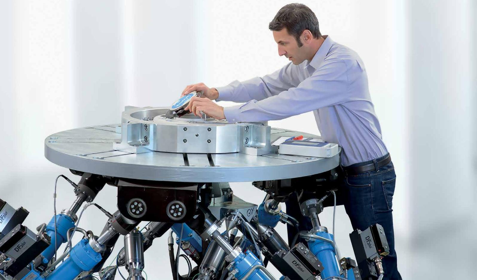
Calibrating a RoadDyn wheel force sensor on hexapod measurement system
