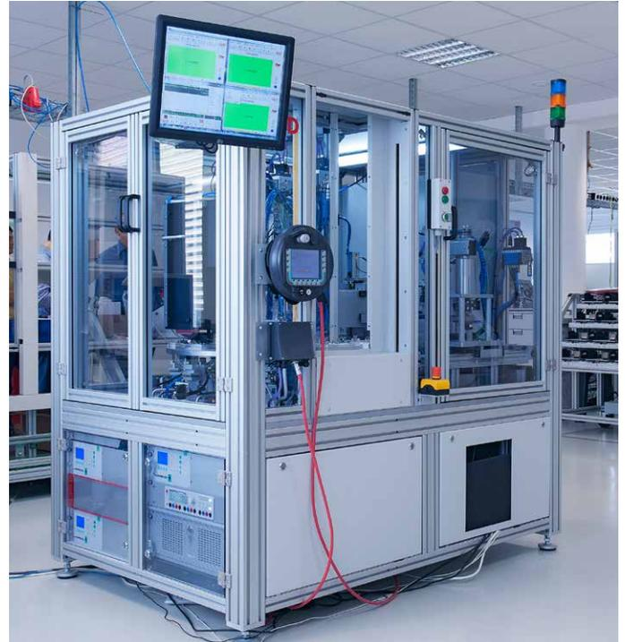
End-of-line test system for electronic components
