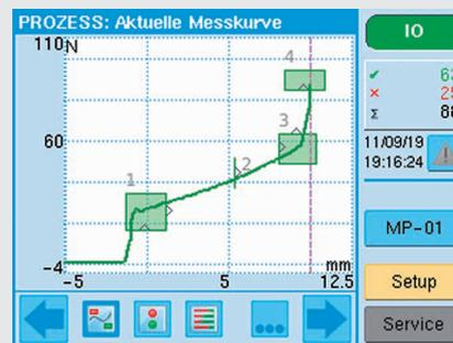
The XY maXYmos monitors oversee and evaluate the quality of a product or production step on the basis of two measured variables in relation to one another
