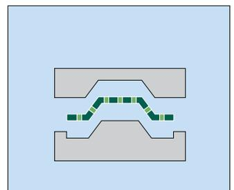
Dry fiber mats or fabrics are impregnated with the resin/hardener mixture.
