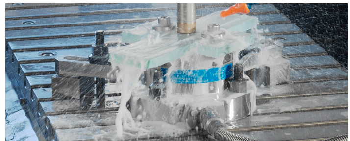
Force measurement during quartz cutting with a Type 9272 dynamometer
