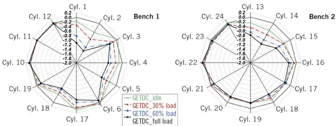
Figure 6: Relative angle position of the GETDC for different loads with respect to the front end at 1,500 min<sup>-1</sup>, optical TDC measurement system
