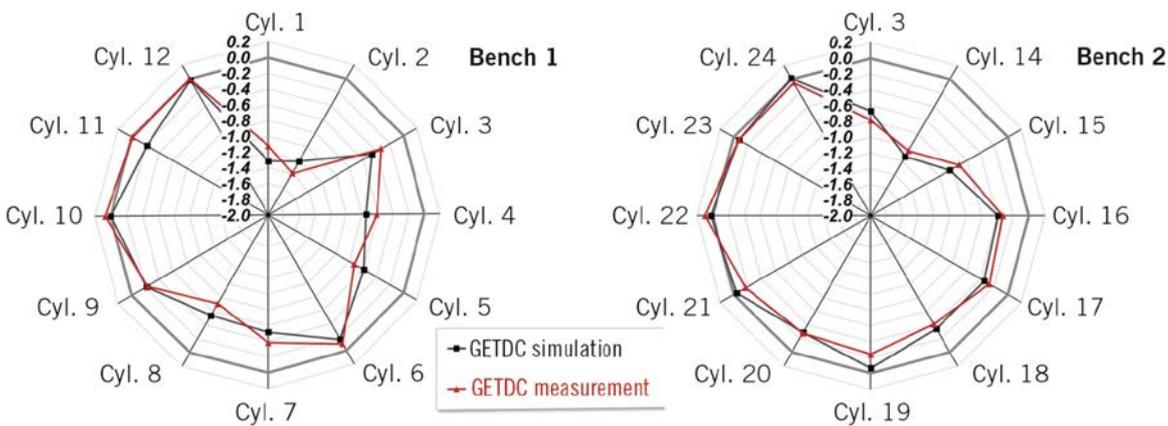
Figure 7: Comparison of determined angle of torsion in GETDC with respect to the front end at 1,500 min<sup>-1</sup> FULL LOAD; simulation vs. optical TDC measurement system
