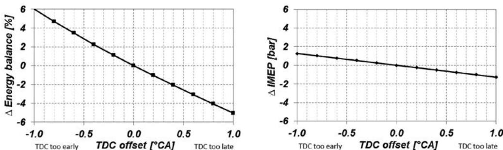
Figure 1: Influence of the crank angle error on energy balance and IMEP
