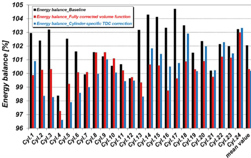
Figure 10: Energy balance for individual cylinders, taking account of differently corrected volume functions at 1,500 min<sup>-1</sup>, full load
