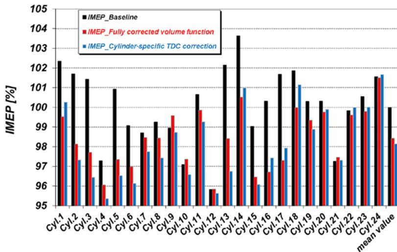
Figure 9: Calculated IMEP, taking account of differently corrected volume functions at 1,500 min<sup>-1</sup> full load
