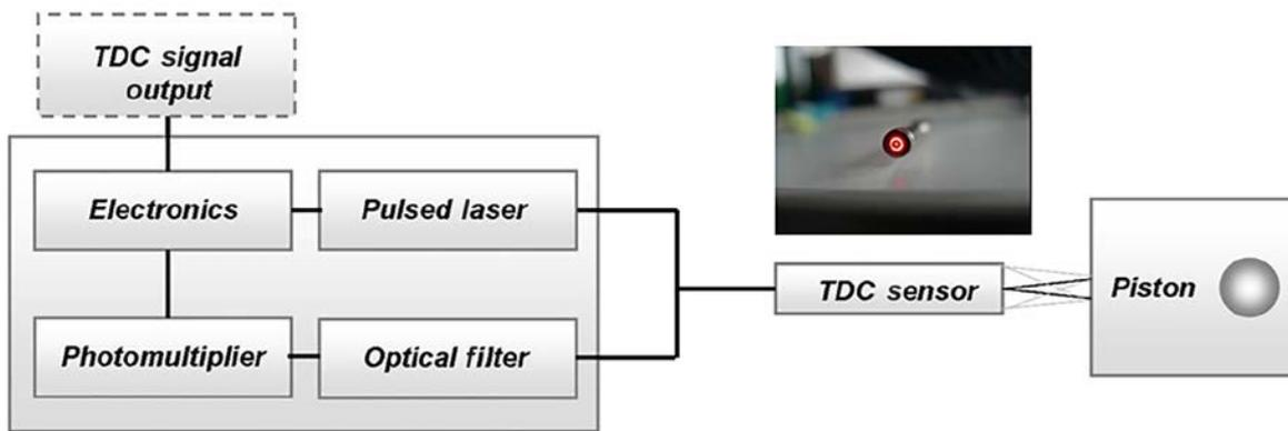
Figure 4: Basic structure of the optical measurement system, incl. frontal illustration of the sensor
