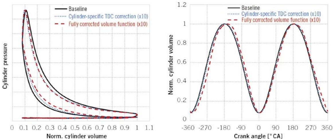
Figure 8: Resulting volume functions: "baseline", "fully corrected volume function" and "cylinder-specific TDC correction"
