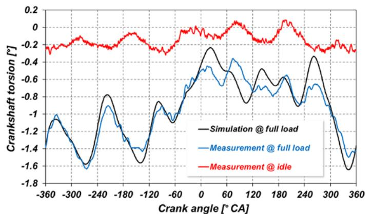
Figure 5: Measured and calculated crankshaft torsion on the flywheel side, with respect to the front end at 1,500 min<sup>-1</sup>
