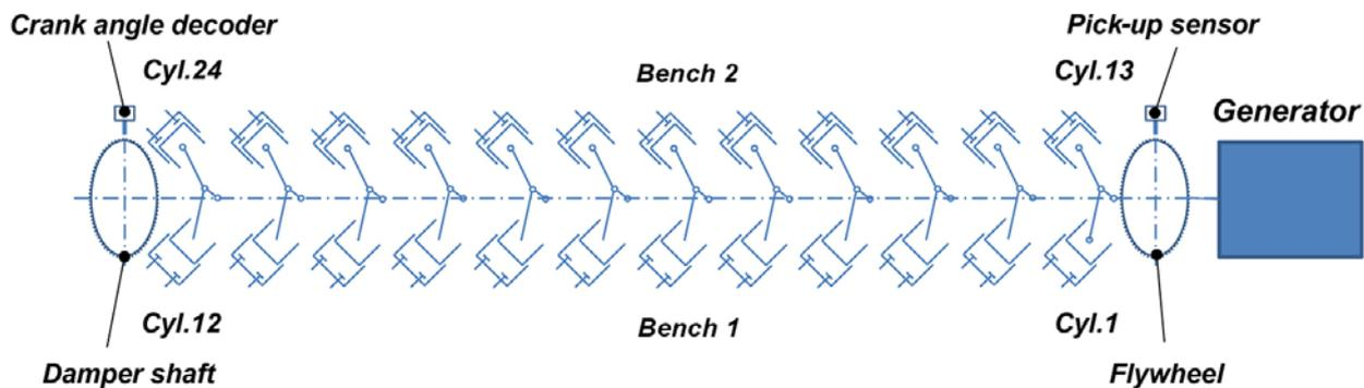
Figure 3: Schematic measuring setup to determine the overall torsion
