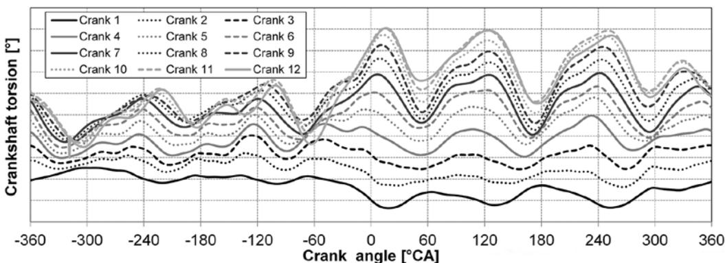
Figure 2: Angle of torsion of individual crankpins relative to a reference point
