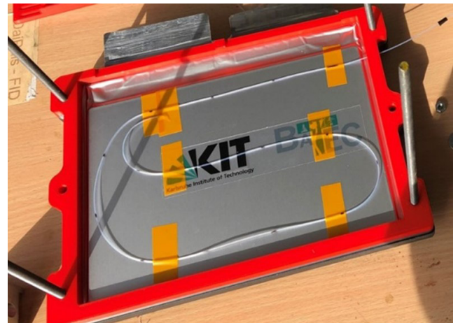
Fig.5: FSI sensor fiber installation on pouch cell
