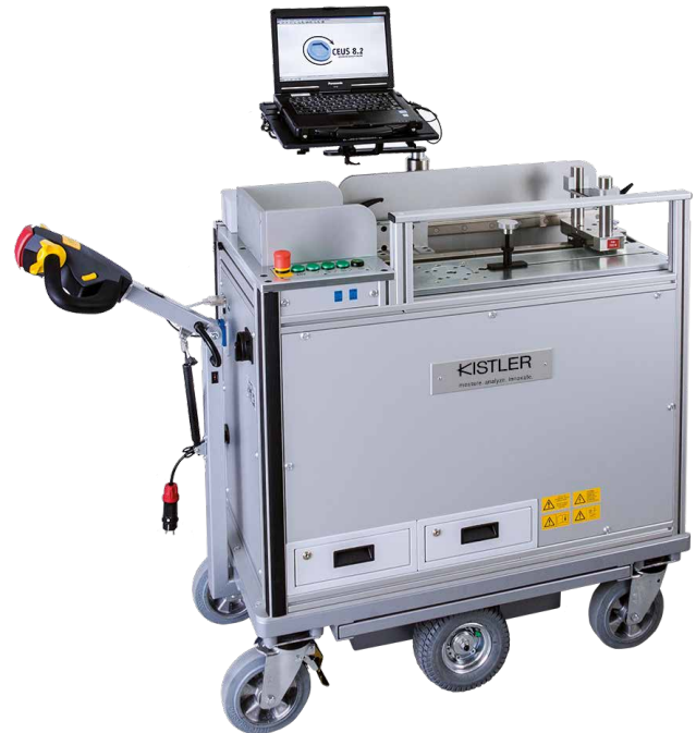
caliTEST mobile 1000/50 with optional propulsion drive and notebook mount
