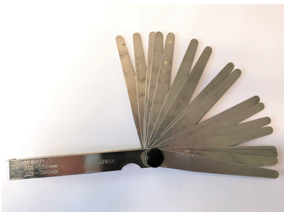
Fig. 18: Commercially available feeler gauge
