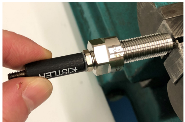
Fig. 17: Adjust the electrode spacing by carefully applying a vertical force
