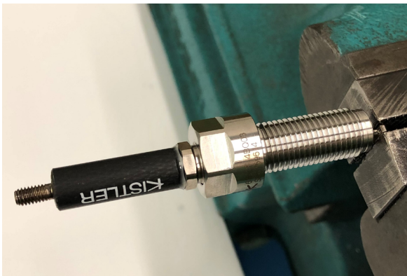
Fig. 16: Adjusting the electrode spacing using a vise – carefully clamp the electrode
