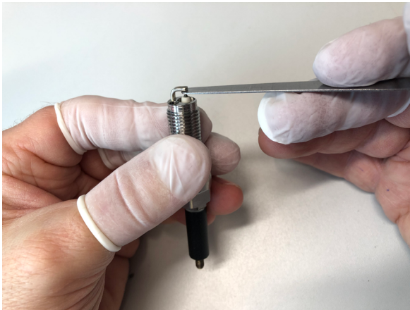
Fig. 14: Checking the electrode spacing with a feeler gauge
