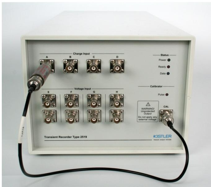
Press button  to start the calibration. The calibration takes approx. 5 minutes.
