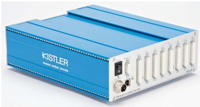
There are (2) 25-pin cables that connect Type 5695... data acquisition box to up to 8 force platforms. The connection to the user's PC (optional) is via the USB cable. Furthermore there is a 9-pin Control I/O input for connection with the adapter box Type 5767. This box allows you to connect other measuring systems (e.g. Visual Systems, EMG) via BNC. In addition, it is possible to interpose the external control unit Type 5233A2 between the force plate and the DAQ system.
