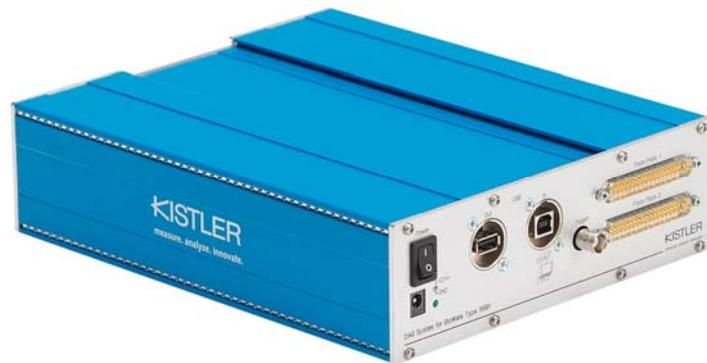
There are (2) 37-pin cables that connect the 5691A data acquisition box to the max. 2 force platforms. The connection to the user's PC (optional) is via USB. Furthermore there is a BNC female connection for an external trigger (trigger in). In addition, there is an USB extension port. To properly connect the cables:
