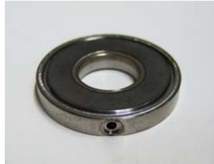
Fig. 10: Cable connection broken off
