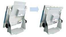
The DIM Cable Extender is inserted at the rear portion of the display. The DIM Cable Extender is supplied with 24 V of power (the display is then supplied by the DIM Cable Extender). The DIM Cable Extender is connected to one or several maXYmos units via an Ethernet cable.
