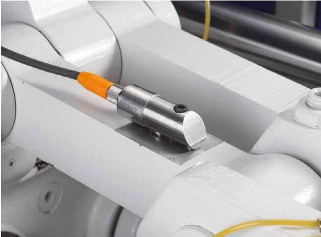
Fig. 8: Indirect force measurement on knuckle joint
