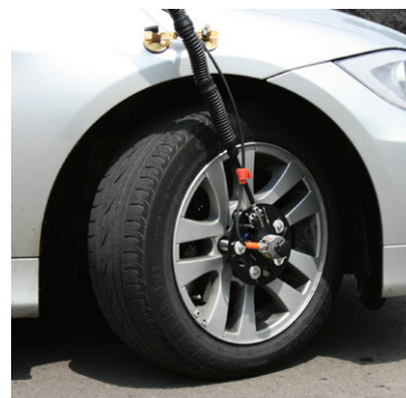
Fig. 2: WPT sensor mounted at the front wheel
