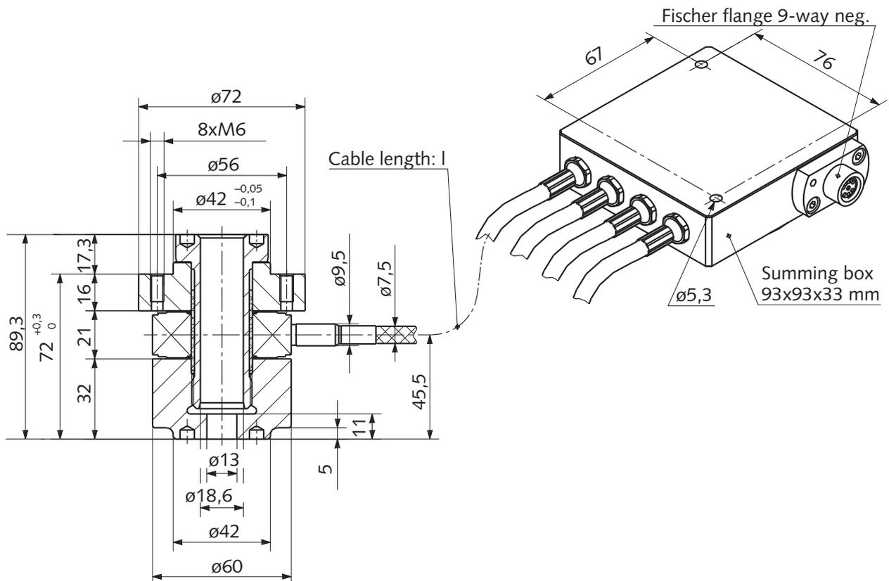
Fig. 2: Dimensions of multicomponent force link set Type 9366CC...
