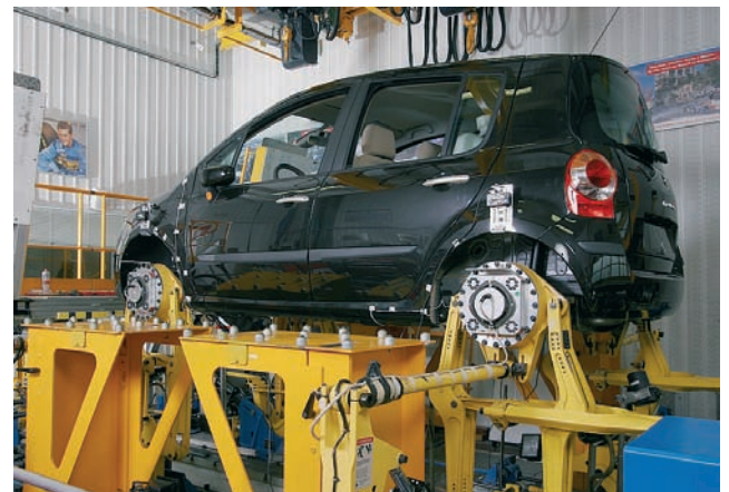
Fig. 2: RoaDyn S625 System 2000 non-spinning on vehicle test stand
