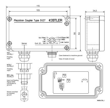
leak-tight connection according to the type of protective cable or a BNC neg. connector. The power input and signal outputs are connected to an 8-pole round connector DIN 45326. Pin assignment is indicated on the case cover.
